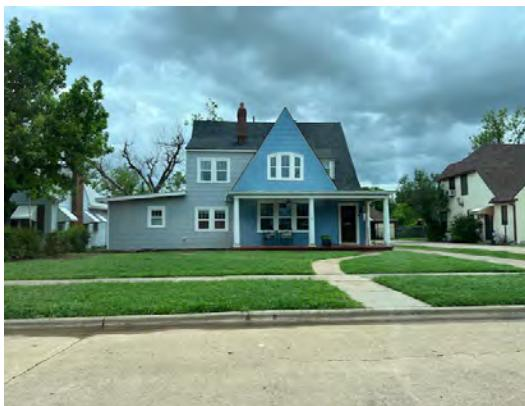
The addition is set flush with the original façade and does not destroy or detract from the character-defining features of the original building. The materials and windows used are in keeping with the original building.
